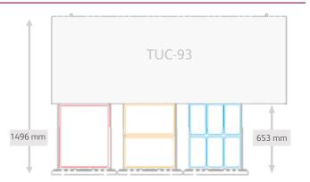
Deep TUC 67 & 93 products are supplied with 1 horizontal divider bar per drawer, facilitating 2x1/1 pans, 6x1/3 pans, or a combination of.
