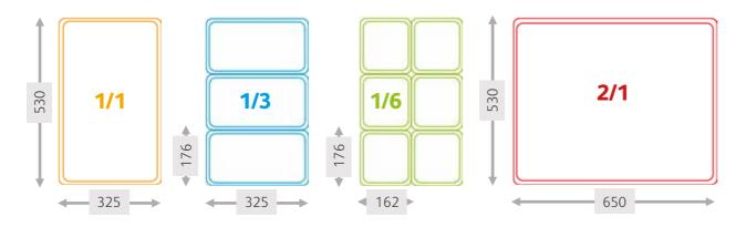
A 1/3 container is 325mm (same as 1/1) but just a third as wide (176mm), while a 1/6 is half the size again. 2/1 is twice the size of 1/1, measuring 530mm x 650mm.
