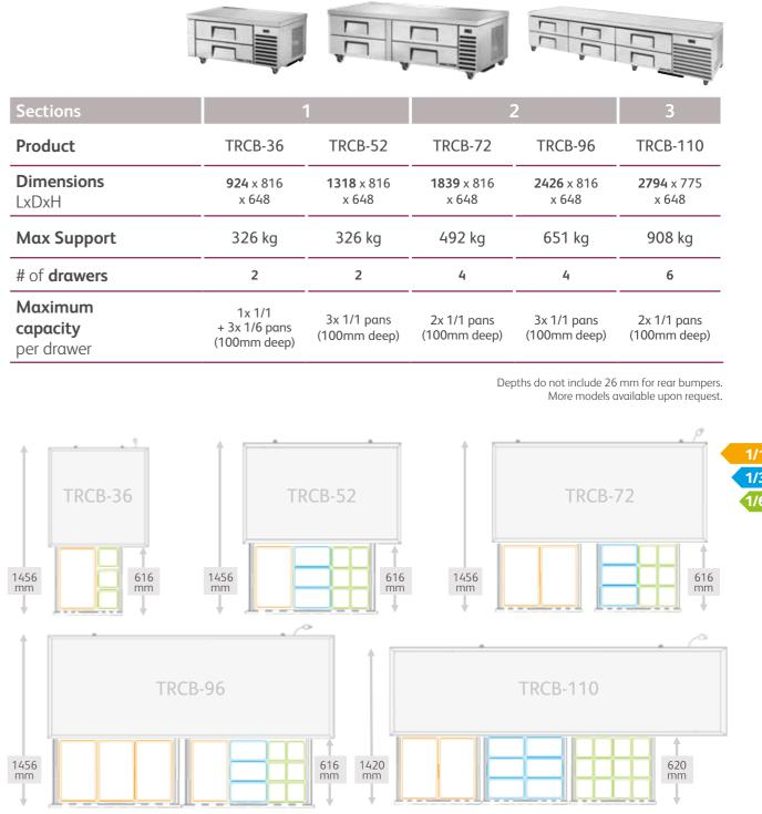
Note: even though drawer capacity of some TRCB units may appear to accept a larger than 1/1 GN pan, the drawer construction of these units are moulded specifically for this pan size as a way of strengthening the drawer and durability of the product.
